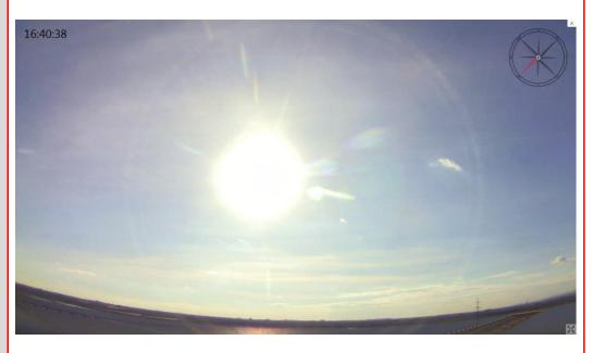
A full cloud camera system was integrated to CSP-FoSyS within another R&D project (WobaS) funded by the German federal ministry for economic affairs and energy, in order to provide a shadow map, to monitor and forecast the shadow movement over the solar field for 15 minutes in advance.
